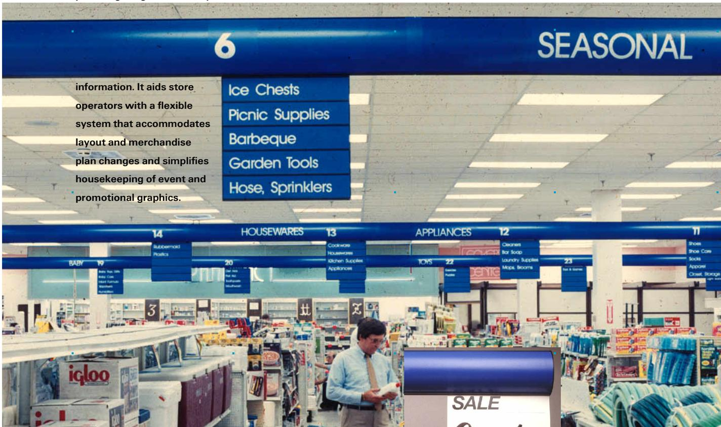
The carrier beam holds department identification and aisle numbers visible at long range. The lower edge of the beam features a key strip from which aisle directories hang and temporary signage like sales promotions and seasonal decorations are conveniently attached and detached. The overall appearance of the store benefits from the visual order the system provides.
